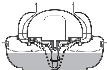
The Condair 505 uses the atomizer principle. The suction piece takes in the water from the reservoir. Then the whirl disk moves the water towards the atomizer ring where it is transformed into aerosol fog.
