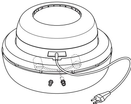
The special version **Condair 505 S** is designed for direct connection to the water supply. The Condair 505 S is equipped with a float valve and a connector for an overflow pipe.
